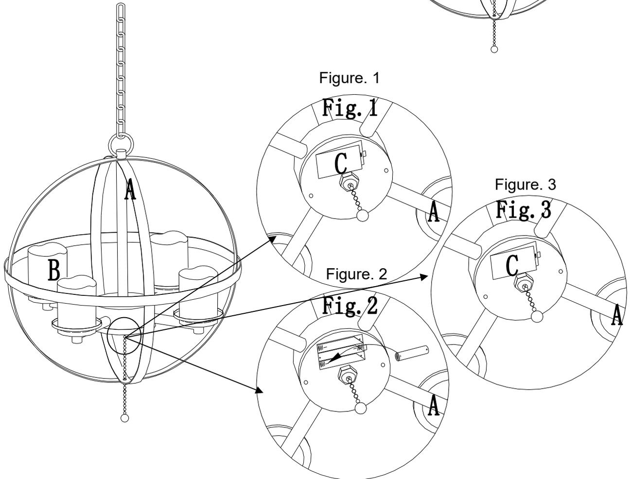
Fig.1: Open the battery cover (C) as shown. / Faites glisser la couvercle du compartiment à piles (C).
