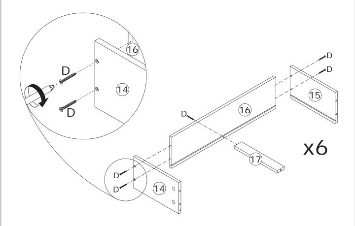
Fix panel 15, 17 and 14 to panel 16 using screw(D) as shown. Insert panel 18 along available grooves as shown.
