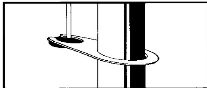
**Curtain clips may have to be re-tightened occasionally due to strong wind gusts. IMPORTANT! Once the legs and cover are assembled, your canopy will act like a kite in the wind. It is imperative that the canopy anchors be installed NOW!**
