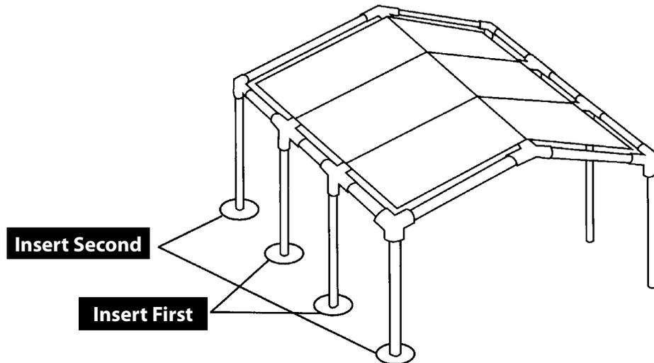
**Step A:** First insert the pipes for the middle poles into the 3- and 4-way connectors, and then connect the end leg pipes in the same way. (See illustration)
