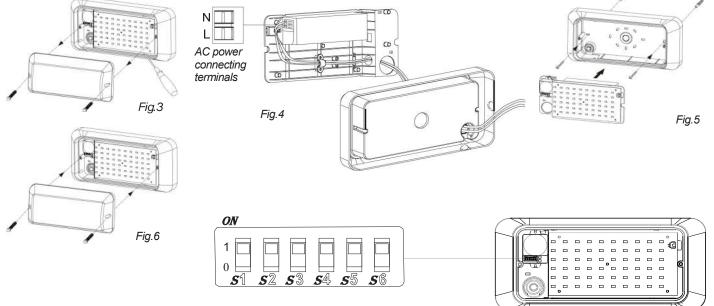
Fig.7 Dip switchs setting reference
