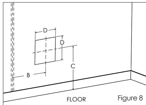
3. Cut the square hole through the wall according to the measurements and positions indicated in figure 7 and 8.
