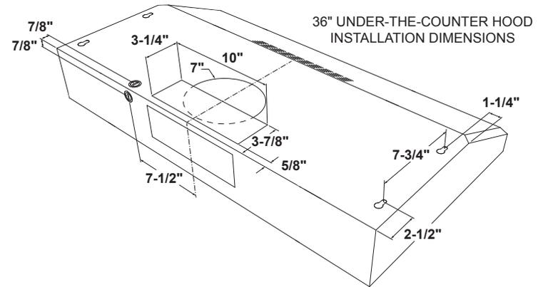
Exhaust outlet connects to 3-1/4" x 10" rectangular duct. Vent top or rear. Includes rectangular damper.
