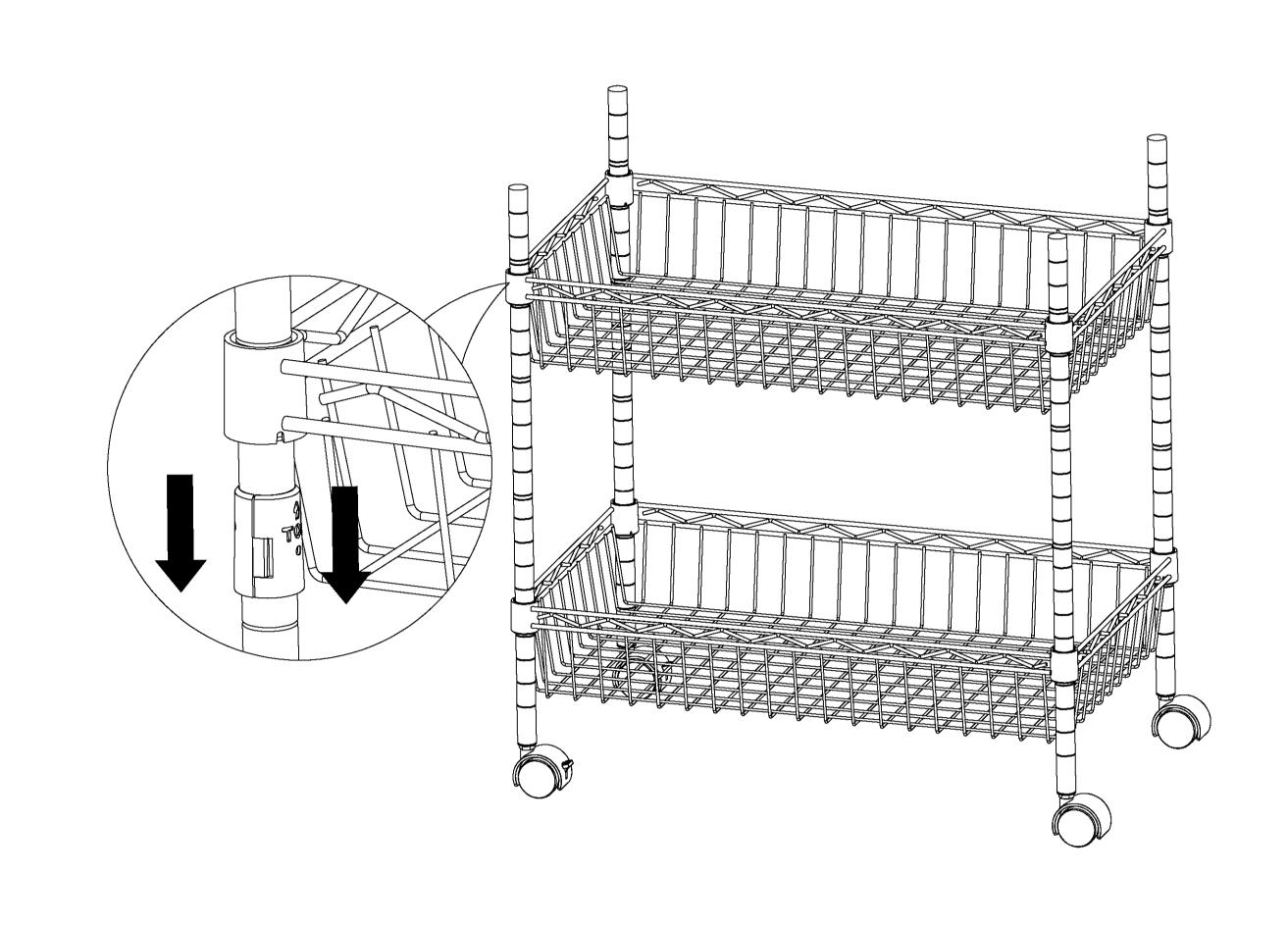
Screw Upper Poles (C) into Lower poles by screw connectors which is already on the upper poles.
