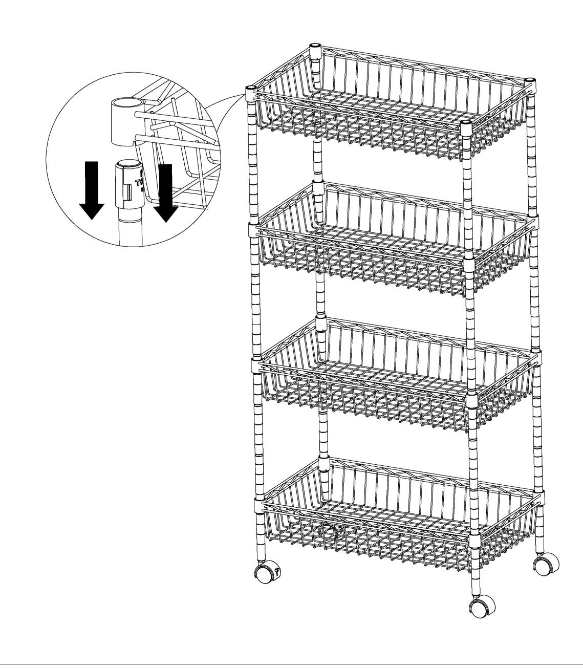
Once all four wire baskets have been installed, pushing firmly down on every basket at corners by rubber mallet to ensure the basket in a place over the plastic clips.
