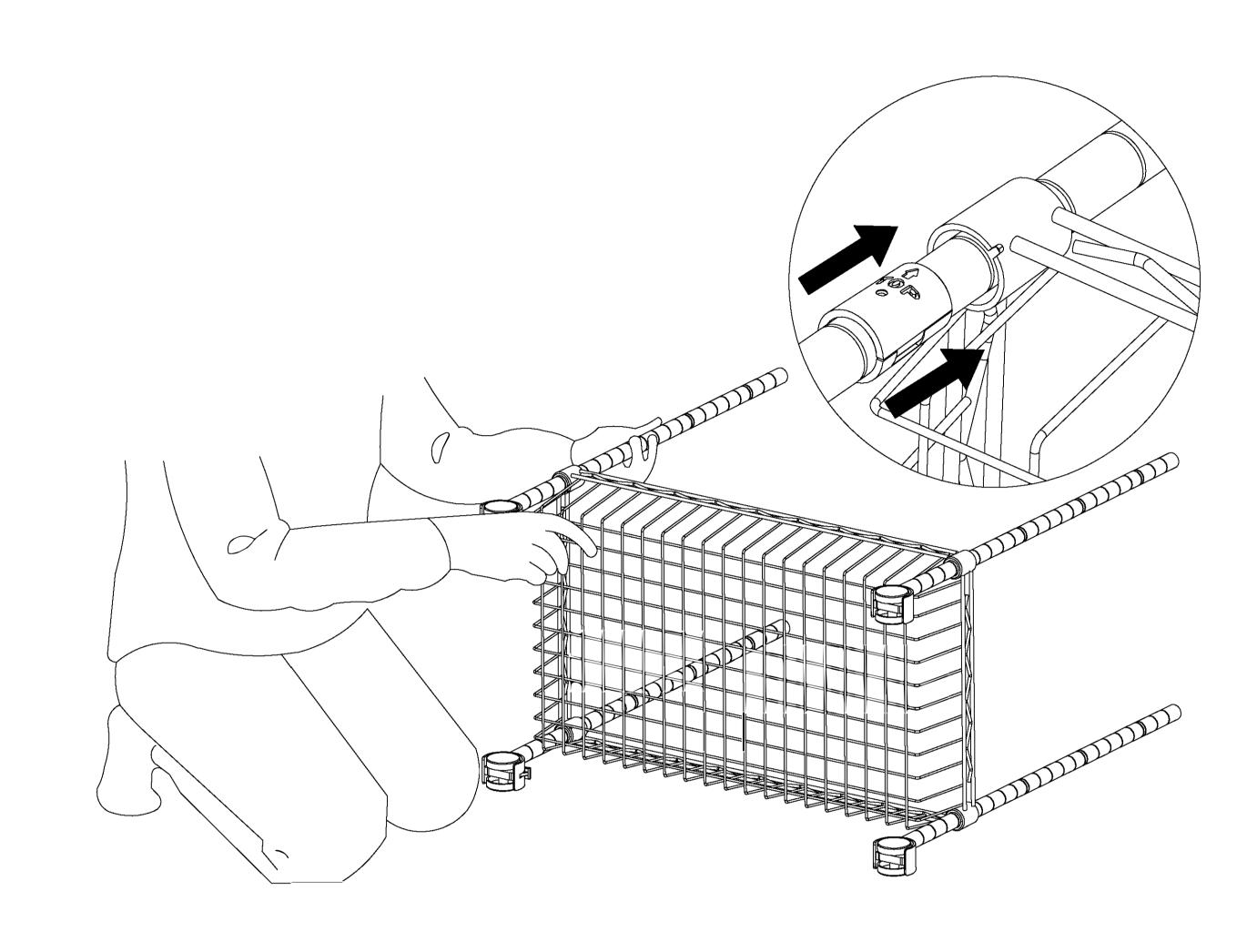
3 Snap plastic clips into the pole grooves of the lower poles at your desired basket height position. Slide down the basket from top down onto the plastic clips.
