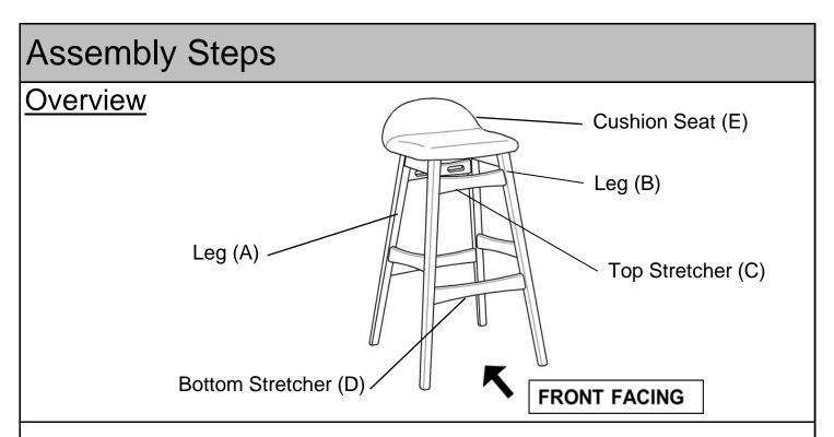
This Bar Stool has multiple parts and may require up to some 30 minutes to assemble. To give you an overview of the Bar Stool parts, the above picture is to help you put the various parts into perspective. Please read through the instructions below to familiarise yourself with the parts and steps before assembly.
