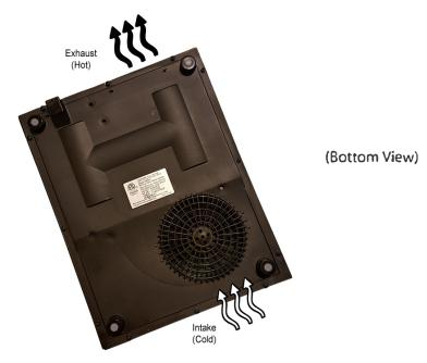
• For proper air circulation, allow at least 3" of clearance from the bottom of the induction cooker to any shelving or storage. The underside of the countertop should not be closed off from the cabinetry underneath for better air flow.
