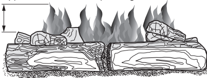
Figure 30 - Correct Burner Flame Pattern with Control Knob Set to HI (5)
