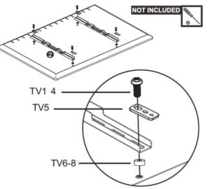
First, make sure the diameter of the bolt (TV1 4) fits your TV. Then, please see the diagram above. You will need to thread the bolt into the TV using the correct washer (TV5) and spacer (TV6-8) if necessary. Please make sure the monitor brackets are vertically centered and level with each other
