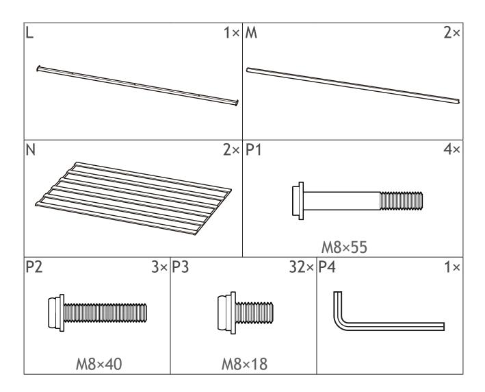
Please do not completely tighten all the hardware, until the entire assembly is complete, unless otherwise indicated in the step-by-step instructions.
