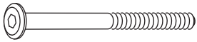
16x 100 mm bolts Used to connect headboards and footboard to side rails
