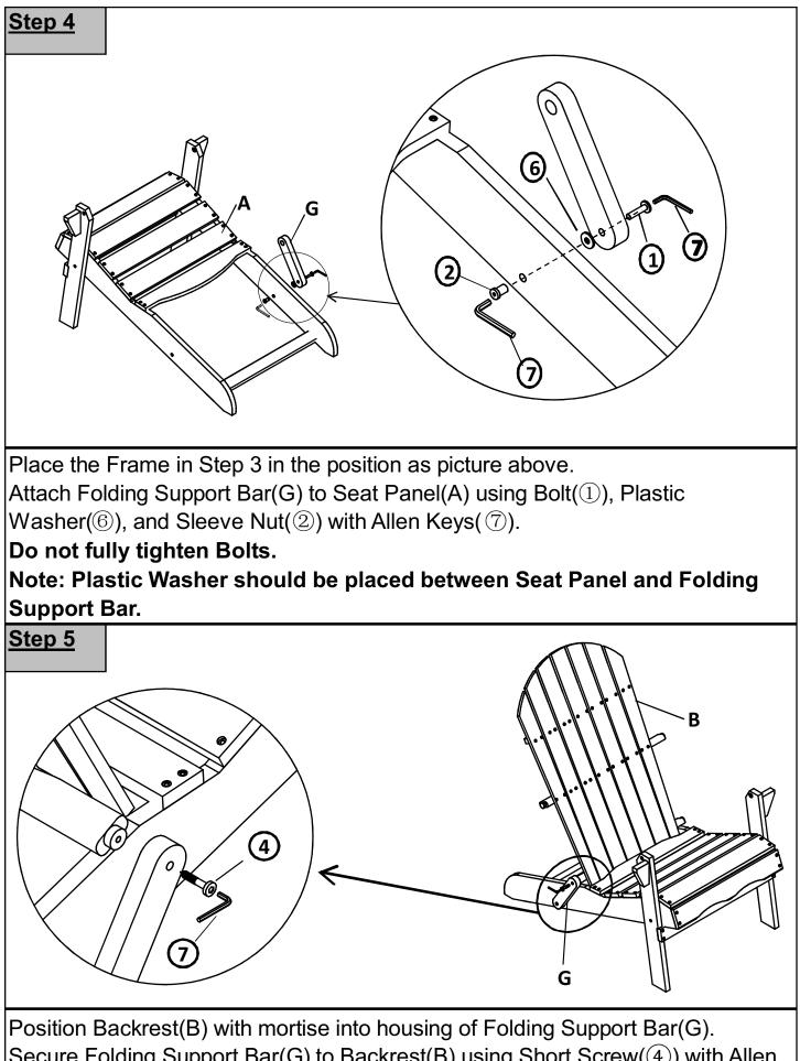
Secure Folding Support Bar(G) to Backrest(B) using Short Screw((4)) with Allen Key((7)).
