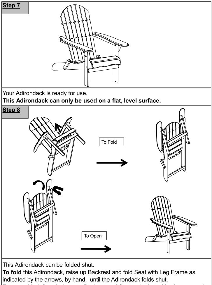
**To open** this Adirondack, open Backrest and Seat as indicated by the arrows, by hand until the Adirondack folds out and locks into position.
