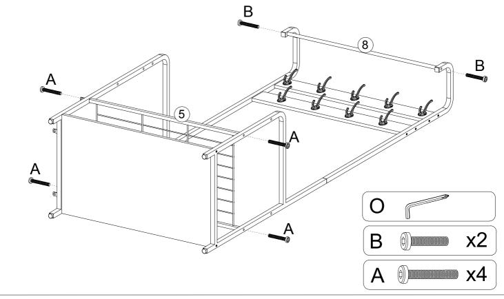
GAUTION: When tightening the screws, tighten sequentially.
