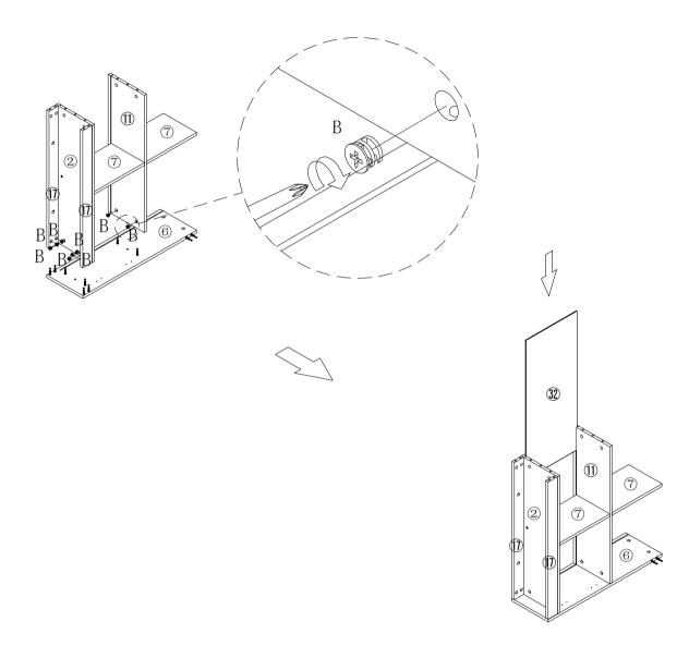
Make sure the arrow on the screw align to the hole on the side.
