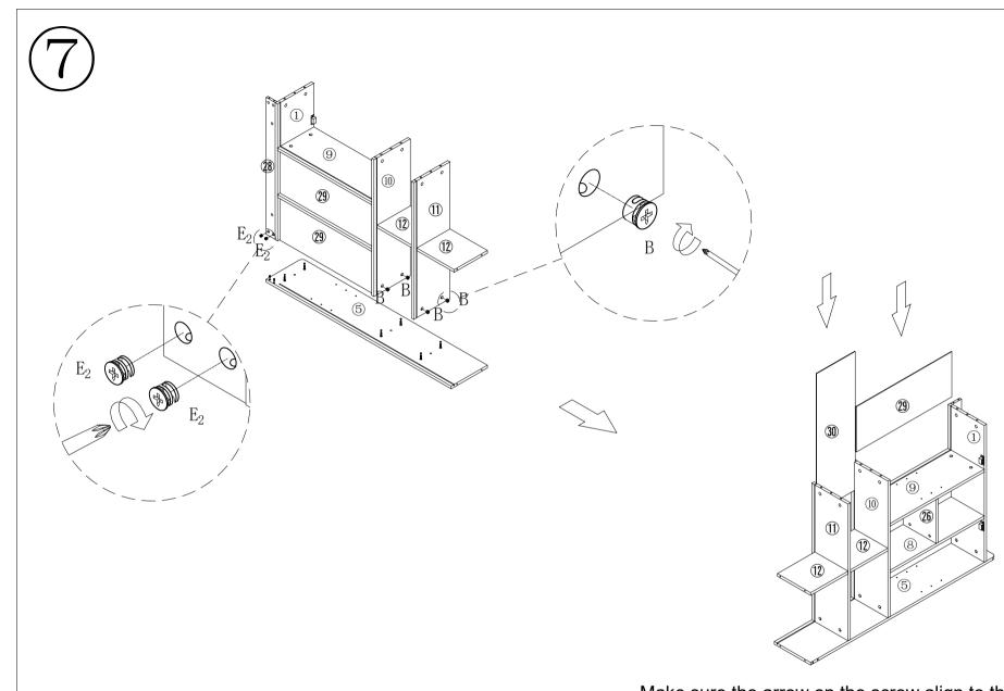
Make sure the arrow on the screw align to the hole on the side.
