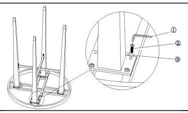
Finally attach Legs(B) to Table Top(A) using Bolts(②) and Washers(③) with Allen Key(①) at the inside mounting positions.
