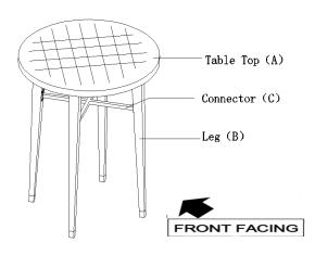
This Table has multiple parts and may require up to 30 minutes to assemble. To give you an overview of the Table parts, the above picture is to help you put the various parts into perspective. Please read through the instructions below to familiarise yourself with the parts and steps before assembly.
