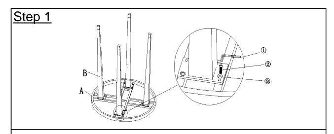
Open the carton and place all the parts onto a clean, non-marring surface. Attach Leg(B) to Table Top(A) using Bolts(2) and Washers(3) with Allen Key(1).
