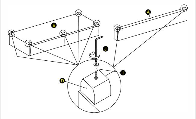
Attach the Footboard Legs (Part D) to the Headboard (Part A) and Footboard (Part B) using seven 70mm Bolts (Part I) and Large Hex Key (Part J). Secure tightly.
