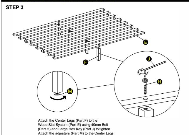
(Part F) and adjust as needed to level the bed.
