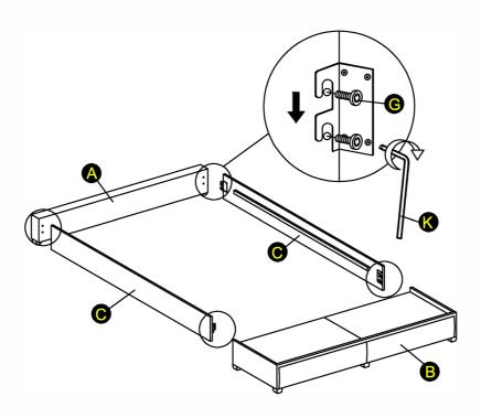
Attach the eight 20mm Bolts (Part G) to the headboard and footboard using the Small Hex Key (Part K). Do not tighten.
