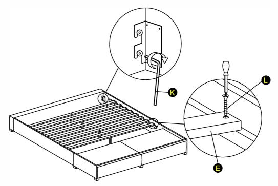
Place the eight slats into the bed as shown. Tighten the bolts on the headboard legs and footboard using Small Hex Key (Part K). Secure the 8 slats using sixteen Screws (Part L) and a Phillips Screwdriver. Your bed is now set up and ready for use.
