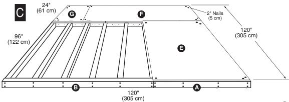
Position Floor Panel 48" x 96" Eflush to the outside edges of Floor Frame. Position Floor Panel 23-7/8" x 96" flush to the outside edges of Floor Frame. Position Floor Panel 23-7/8" x 23-7/8" flush to the outside edges of Floor Frame. Secure panels with two 2" nails at outside corners and one 2" nail at other corners.
