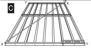
**C:** Completed Floor Frame should be positioned at building site, leveled, using shims between floor frame and ground before proceeding to Floor Panel Attachment.
