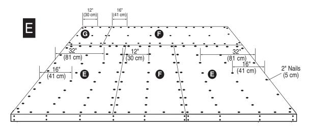
Nails every 12" (30 cm) through Floor Panels into all Floor Bond Boards and Floor Joists
