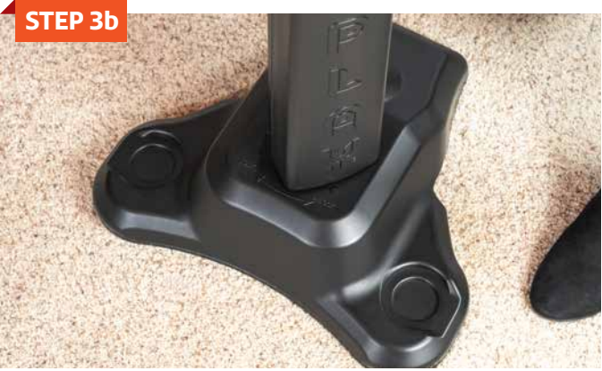
Insert the post into the base. Insert the post into the base and turn clockwise 90° until it locks into place.
