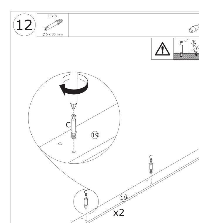
Insert quickfit screw(C) into corresponding holes in plate 19 with a screwdriver as shown.
