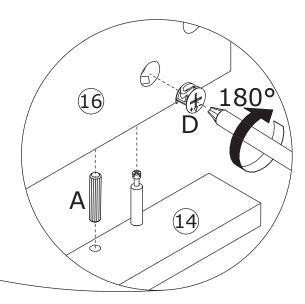
Attach plate 15 to plate 14 with wooden dowel(A), put cam lock(D) into holes in plate 15 and turn clockwise to tighten as shown.
