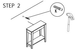
1. Use a light hammer to tap anchor into hole. 2. Anchor should fit snugly. If hole is too small, drill again to increase hole size . Do not force anchor into wall.
