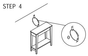
1. Insert strap thru bracket attached to wall. then thru bracket on item, and into head of strap. 2. pull lightly til strap stops.
