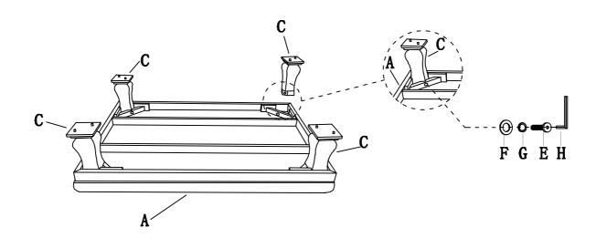
Attach bottom(B) to leg(C) by using screw(D), flat washer(F), spring washer(G) and allen wrench (H) as shown.
