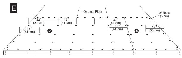
Nails every 12" (30 cm) through Floor Panels into all Floor Bond Boards and Floor Joists
