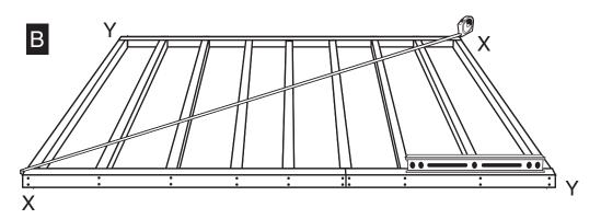
**B:** Completed Floor Frame should be positioned at building site, leveled, using shims between floor frame and ground before proceeding to Floor Panel Attachment.
