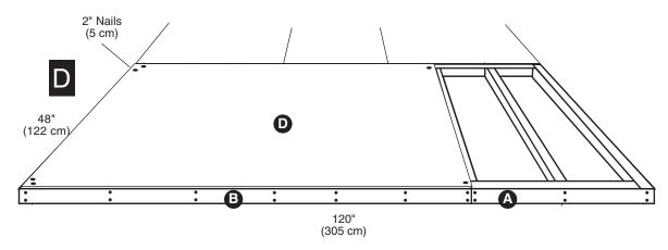
**D:** Position a 48 x 96" Floor Panel **D** flush to the outside edges of sides and back of Floor Frame. Secure panel with two 2" nails at outside corners and one 2" nail at other corners.
