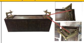
2. Align Pre Drilled Holes From Top[partT] With Pre Drilled Holes From Leg[partL] Matching "A" with "A" And "B" with "B". Then Secure The Leg[partL] With Top Using Allen Bolt[part H1] And Washer[part H2]. Finger Tighten Allen Bolts Clockwise Direction And Do Not Fully Tighten Until Stretcher Is Assembled.
