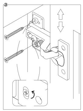
To adjust the door vertically loosen the screw as shown and move up and down as needed.
