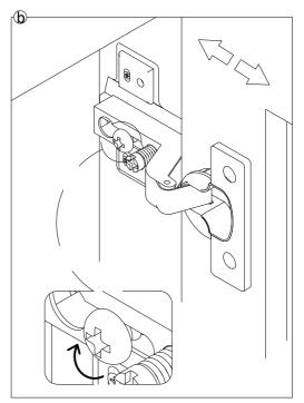
To adjust the gap from the door to the main frame turn the screw clockwise or anticlockwise as needed.
