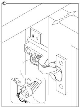
To adjust the door laterally ( such as changing the gap between the two doors), please adjust the screw as shown by turning clockwise or anticlockwise.
