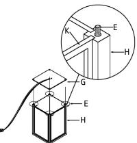
Pull the socket and cord through socket board G's hole and turn to tighten. Then, insert the stud bolts **(E)** into the board and into the short poles **(H)** and screw tight.
