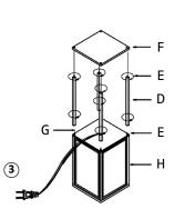
Screw four long (D) poles and (F) shelves together with the (E) screws until tight. Repeat this step to build another level.
