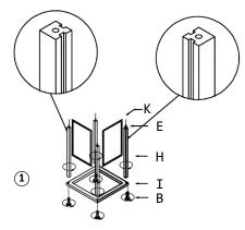
Place frame (I) on a flat surface. Insert four (B) screws into the frame and into the short poles (H) and screw until tight. Then slide the shades (K) into the short poles.
