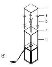
Screw four long (D) poles and (F) shelves together with the (E) screws until tight. Repeat this step to build another level.
