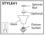
STYLE#1 - Remove spinner nut from socket. Position glass on the fixture and secure with spinner nut. Install proper bulb type and wattage. Note: Glass may face up or down.
