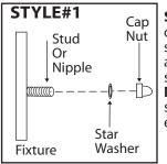
STYLE#1- Tuck electrical wires into outlet box and position fixture over studs or nipple on mounting bracket assembly. Secure fixture in place with star washer(s) and cap nut(s). Note: If required, assemble body and spread the arms of the fixture out evenly.
