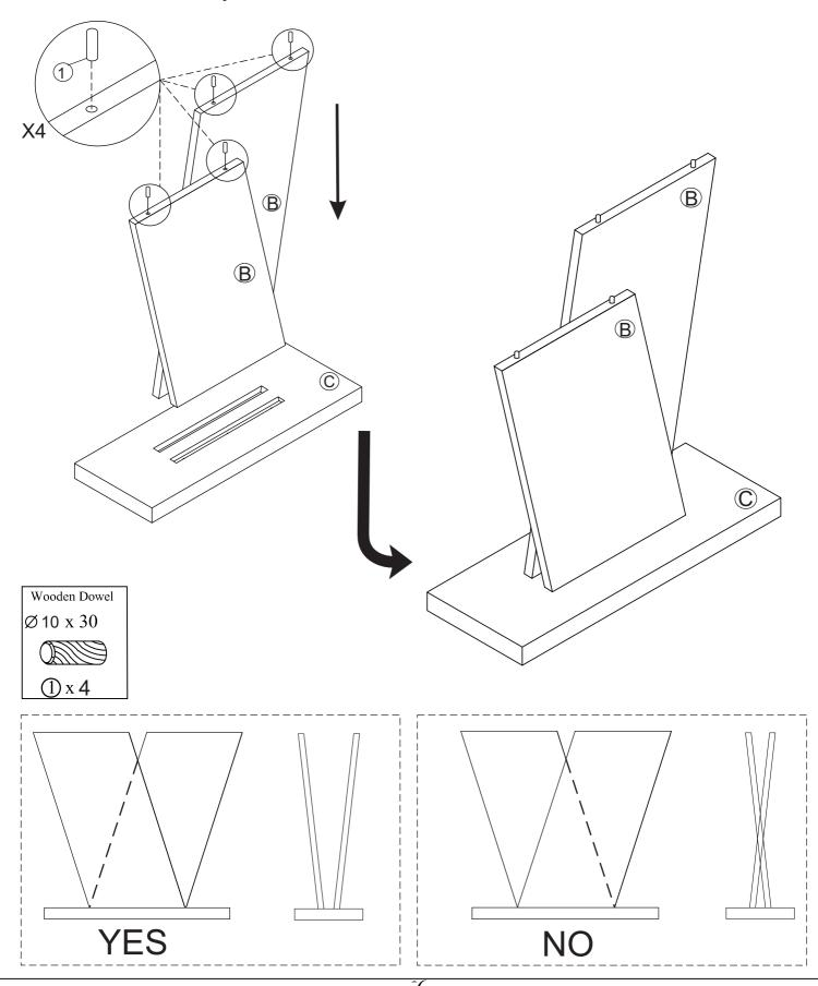
$Step \ 2 \ {\tiny \ \ Next, \ attach \ the \ Support \ Legs \ (2) \ to \ Legs \ (B), \ Align \ hole \ with \ Wooden \ Dowels \ (1)} } \ and \ Wood \ screw \ \emptyset \ 4 \ \times \ 45 \ (3). \ Tighten \ to \ 100\%$
