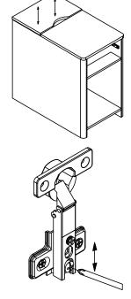
1. The screws can be loosened to adjust the uneven problem under the table top.
