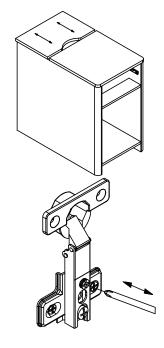
2. Adjust the screws shown in Fig. 2 and pull the door backand forth so that it can be opened smoothly.
