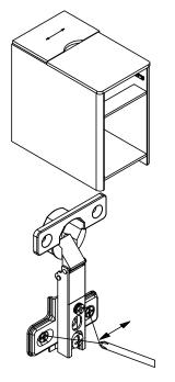
3. Adjust the screws shown in Figure 3 to adjust the door leftand right to the right position.
