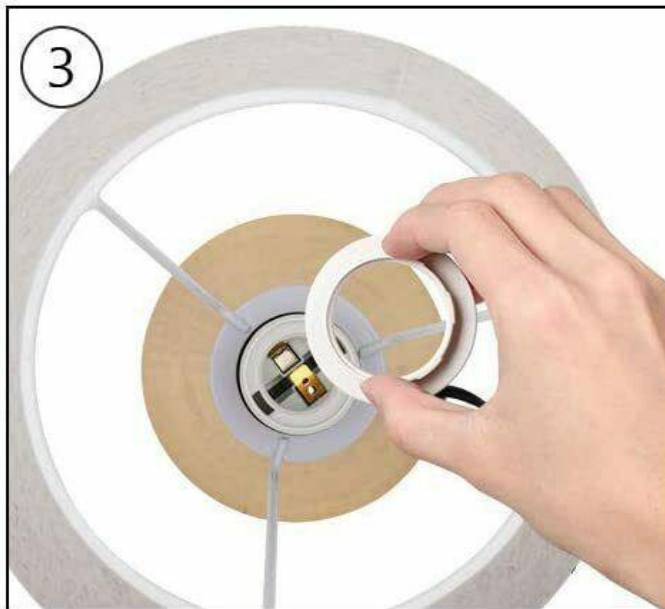
Tighten the fixing ring
