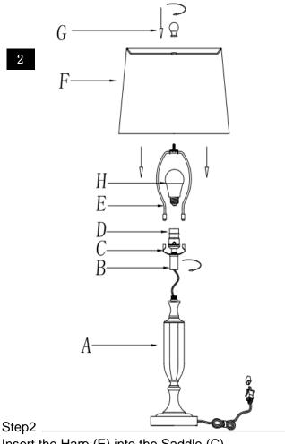
Insert the Harp (E) into the Saddle (C). Put the shade(F) on the Harp(E),then tighten the Finial (G)into the Harp (E) Insert the bulb(H) into the socket(D).
