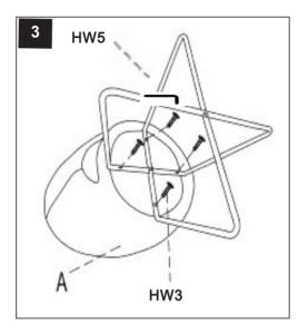
Step 3 Put the frame in the bottom of seat(A) Hex bolts(HW3)
