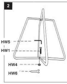
Step 2 Assemble the bottom of frame for using Allen key(HW5) with Gold Flat Hex bolt(HW1) Then use the Allen key(HW5) with Then lock the Hexagon Wrench(HW6) with Flange(HW4)
