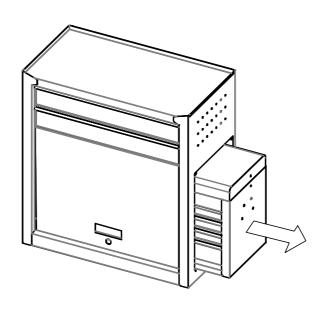
Step 4 Install side panel with screws "E".
