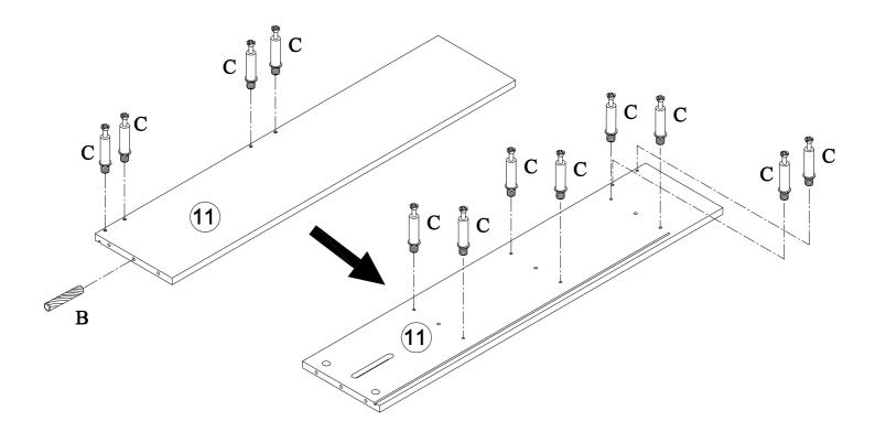
I.Screw in cam-bolt (C) into the designated holes on panel (10,12). II.Insert wood dowel (B) to panel (10,12).
