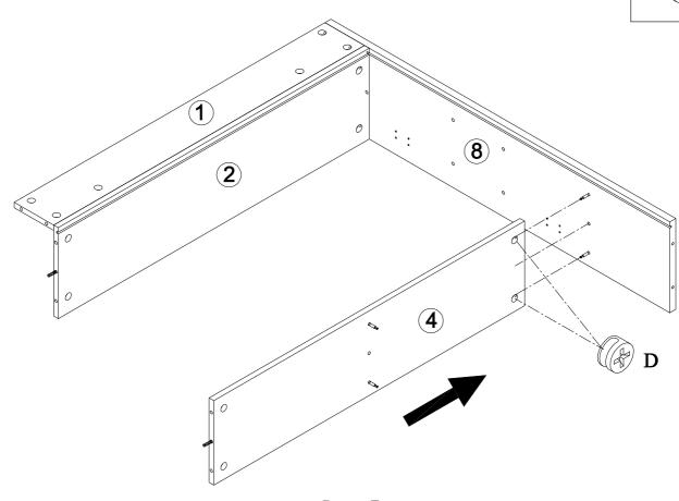
I.Attach panel (8) on to panel (2,4), insert cam-lock (D) into the holes on panel (2,4), then turn clockwise to lock onto cam-bolt.
