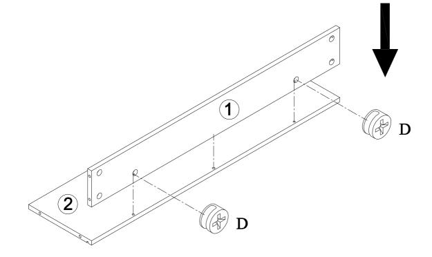
I.Attach panel (8) on to panel (1,2), insert cam-lock (D) into the holes on panel (1,2), then turn clockwise to lock onto cam-bolt.
