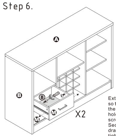
Extend the two outer slides of the runners so that they could align with the sides of the drawer. Make sure the pre-drilled holes from the drawer align with the screw holes of the outer slides. Secure two screws from the inside of the drawer using a Phillips screwdriver to tighten them to the outer slides.
