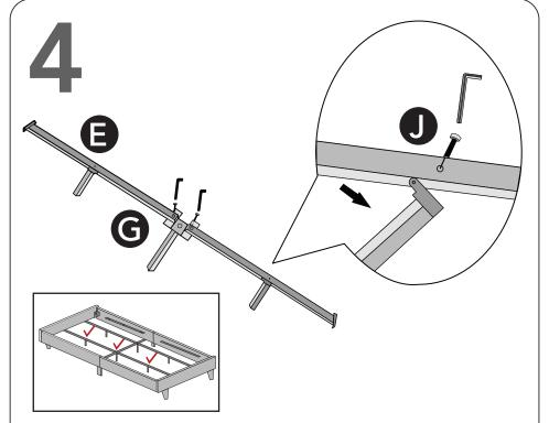
PARTS REQUIRED: Center Support Rails, U-bracket, Bolts
