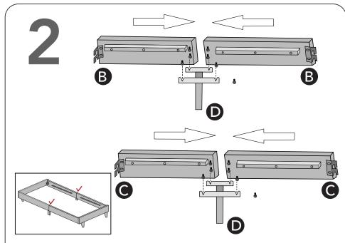
PARTS REQUIRED: Left & Right Side Rails, Horizontal Support Rail
