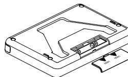
Insert supplied batteries and close battery cover
