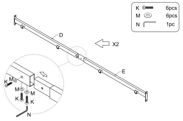
Assemble the side rail (D & E) to the extension leg (C) and the footboard (B) with 4pcs bolts (I), 4pcs bolts (K), 4pcs nuts (L), and 8pcs flat washer (M), then fastened using allen wrench (N) and wrench (O).
