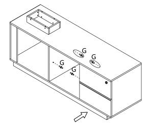
Install G (for placing divider) in position shown
