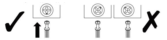
When screw A and screw B are connected, refer to the example for the correct starting position of B
