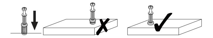
When inserting screw A into the screw hole, it should be perpendicular to the panel and hammered into the shoulder position with a small hammer, taking care not to be too tight or too loose
