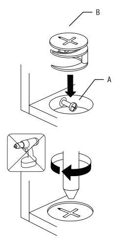
When the two panels are linked through A and B, pay attention to: A screw needs to be inserted into the slot of B card, adjusted to the correct position, and then rotated clockwise to lock (the two panels can be linked tightly).
