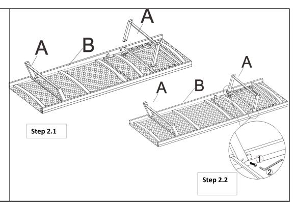
Attach Legs(A) to Seat Panel(B) using Bolts(1) with Allen Key(2) as shown above. **Do not fully tighten the Bolts.**
