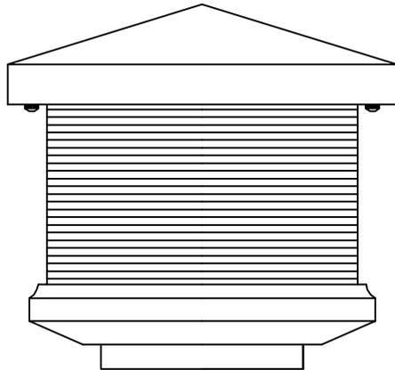
To prevent water intrusion, caulk around post cup where fixture meets the wall using outdoor silicone sealant.
