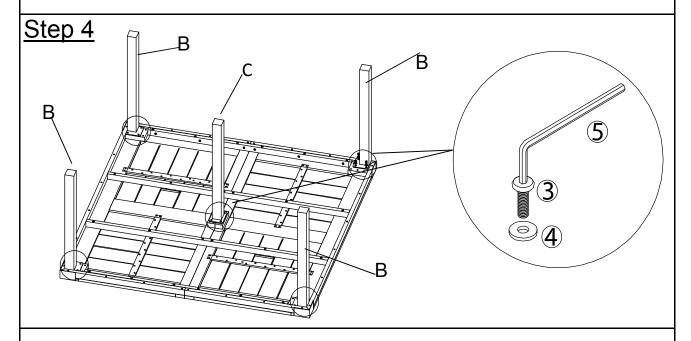
Attach Legs(B) and Support Leg(C) to Foldable Table Top(A) using Bolts( $\mathfrak{F}$ ) and Washers( $\mathfrak{F}$ ) with Allen Key( $\mathfrak{F}$ ) as shown in picture above.
