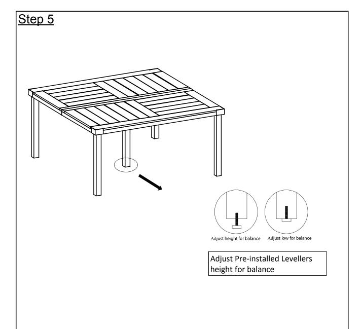
Place the Table onto a flat, level surface.
