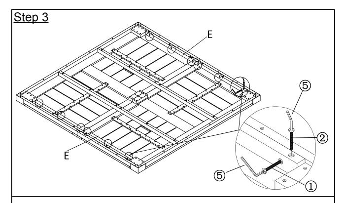
Attach Second Suppor Bars(E) to Foldable Table Top(A) horizontally using Bolts( $\widehat{\mathbb{1}}$ ) with Allen Key( $\widehat{\mathbb{5}}$ ) and vertically using Bolts( $\widehat{\mathbb{2}}$ ) with Allen Key( $\widehat{\mathbb{5}}$ ) as pictured above.
