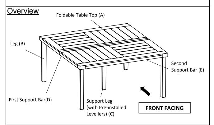
This Table has multiple parts and may require up to 30 minutes to assemble. To give you an overview of the Table parts, the above picture is to help you put the various parts into perspective. Please read through the instructions below to familiarise yourself with the parts and steps before assembly.
