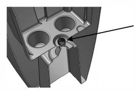
For indoor use, press the red plug down firmly into the overflow drainage hole to seal the planter before use.
