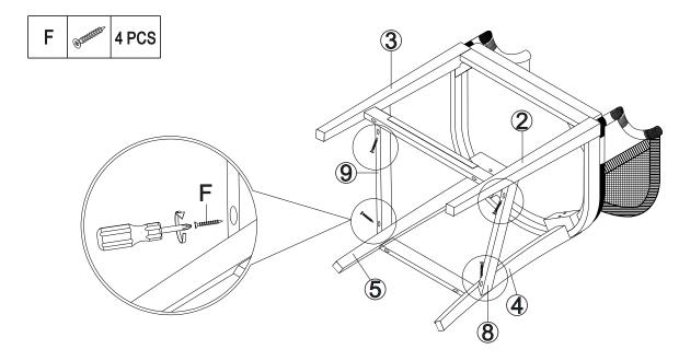
FULLY TIGHTEN ALL SCREWS, THEN FULLY TIGHTEN ALL BOLTS
