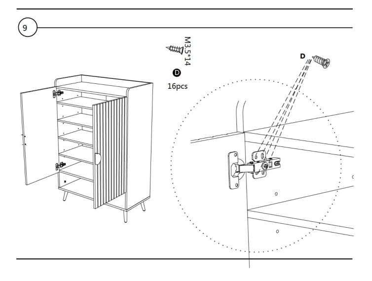
If there is misalignment after you install, adjust the screw to the best condition
