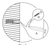
Step 4 Attach wall mount to the wall stud
