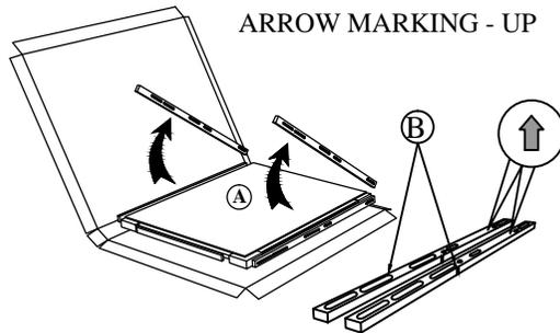
**STEP 2 :** Align & fasten mirror support (B) to the back of mirror (A) using short JCBC bolt(1),spring washer (3) & flat washer (4). **DO NOT FULLY TIGHTEN AT THIS STEP.**
