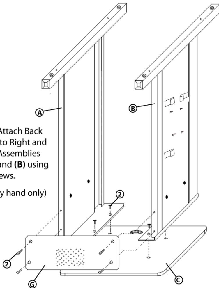
**Step 1B:** Attach Back panel (G) to Right and Left Side Assemblies parts (A) and (B) using 4 # (2) screws.
