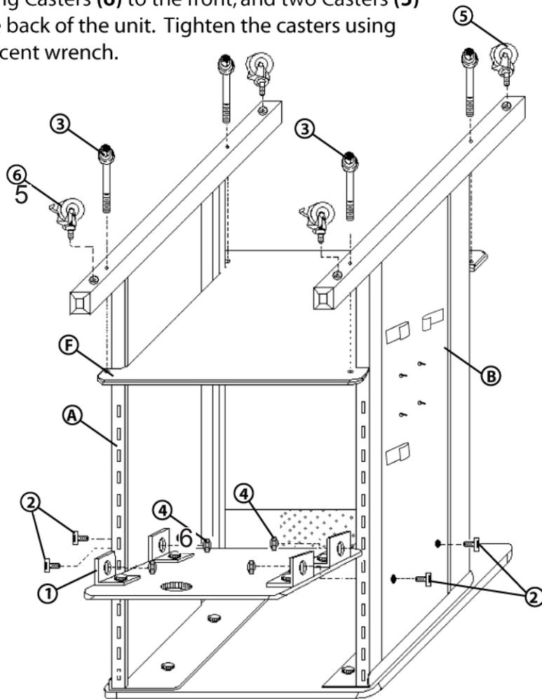
**Step 3B:** Slide Middle Shelf (E) Between Right and Left Side Assemblies (A and B) and attach using 4 # (2) screws and 4 # (4) nuts as shown above. Tighten all screws well using the Allen wrench.
