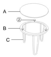
Carefully place the Tempered Glass(A) on the Table.
